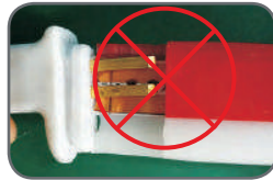
Pin shift may cause short circuit
