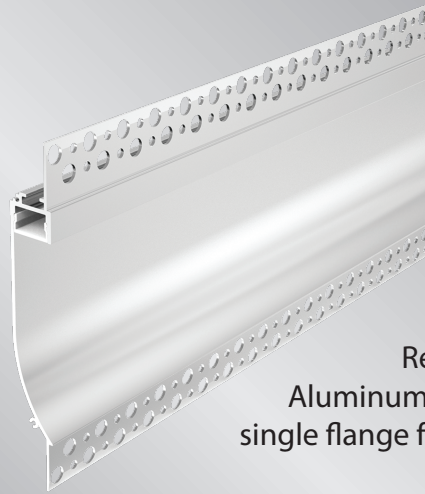
AP-85 98" x 4" Indirect Recessed trim-less Aluminum LED Profile with single flange for 5/8" drywall, wall to ceiling or ceiling to wall. Also can be used as a baseboard
